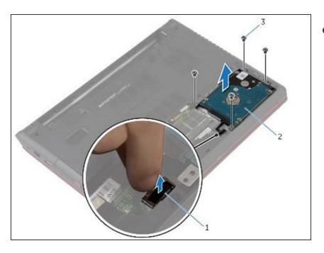
Connect the hard-drive cable to the system board.
