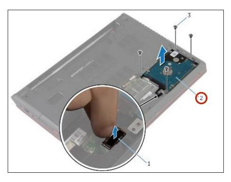
Gently lift the hard-drive assembly out of the computer base.
