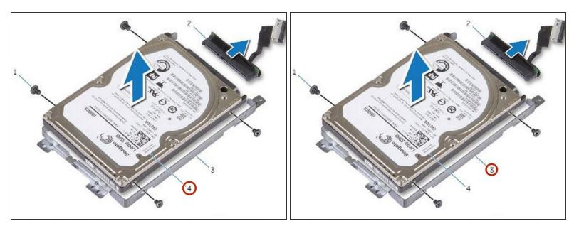
• Lift the hard drive out of the hard-drive bracket.
