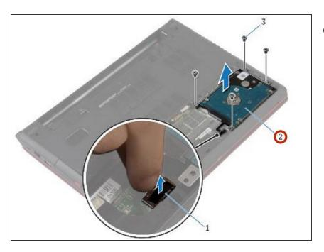
Place the hard-drive assembly into the hard-drive bay.
