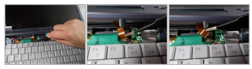
Use the tweezers to disconnect the ribbon cable from the motherboard.
