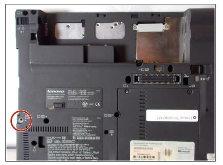
First flip the device so its bottom side is face up. and locate the Philip #00 screw that is marked in the image.
