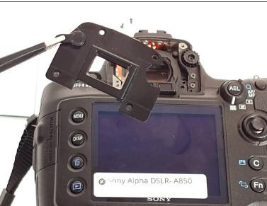
Grasp the side of the window with either a set of tweezers or your fingers. Lift upwards and slightly towards the base of the camera.
