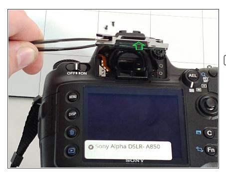
To reinsert the window, push inward and slightly forward. There is a tab on the camera that the window must catch on in order to be put into place.
