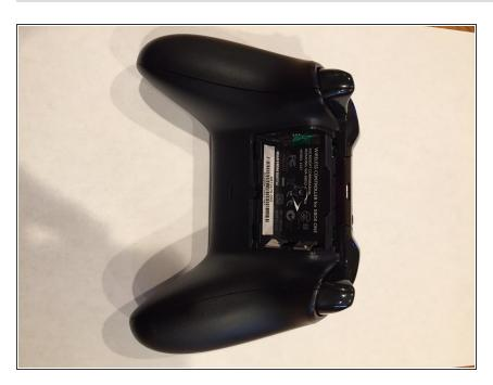
Remove the battery cover and batteries.
