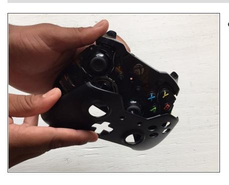
After removing the screws the front panel should come off easily.
