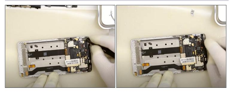
• Use a pair of tweezers to remove the small metal piece from the top of the motherboard.
