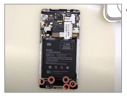
• Use a Phillips screwdriver to remove the five screws in the plastic covering at the bottom of the device.
