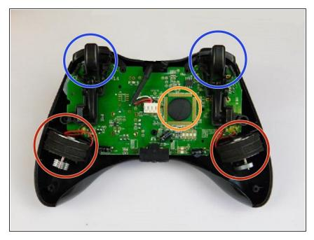
• In the back, you will see the vibrator motors (Red) in the controller handles. You will also see the shoulder buttons (Blue) and the controllers central "Hub" where all the power is stored (Orange).
