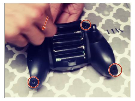
The first thing you want to do is to turn over the XBox controller and locate the 4 screws on the back.
