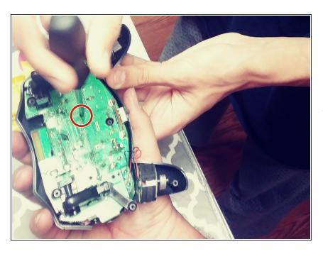
You will be looking at the controllers circuit board. There will be another screw in the middle of the board that you would want to take out as well. It's a different type of screw from the ones on the back cover, so separate that screw and the ones from the back cover.
