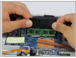
Locate the RAM. The RAM will be covered by a black protective plastic. Once it is located, the
