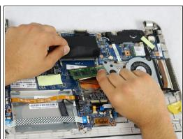
On the ends of the RAM, there are small clips. Click the small clips by pushing them away from from the RAM. Once the RAM has been clicked off gently pull out and remove.
