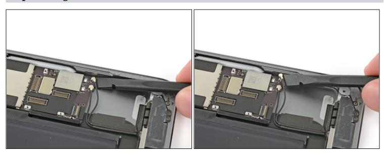
• Insert a spudger under the antenna cable closest to the edge of the iPad and lift upward to disconnect the antenna cable connector.
