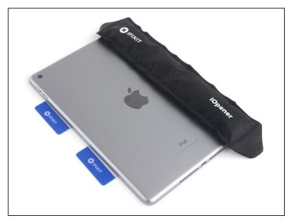
Place an iOpener on the right side of the battery, opposite the cards, to loosen the adhesive.
