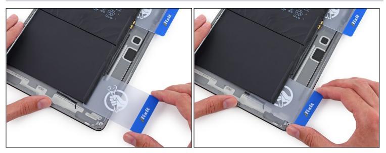
• Place a second plastic card about halfway under the left hand battery cell to prevent it from readhering when you reapply the iOpener.
