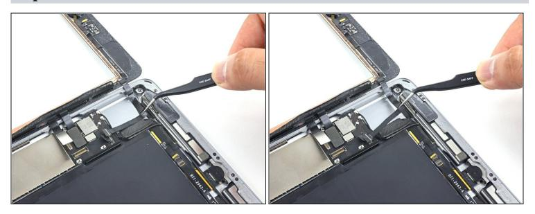
• Carefully peel the home button ribbon cable up off of the adhesive holding it to the rear case.
