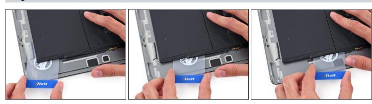
With the card roughly halfway inserted, slide it toward the top of the iPad, stopping before the battery contact post.
