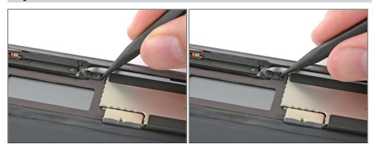
• Use the pointed end of a spudger to flip up the retaining flap on the upper button assembly cable connector.
