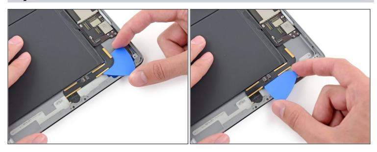
Continue to slide the opening pick under the cable, stopping before the cable bends to the Lightning connector.
