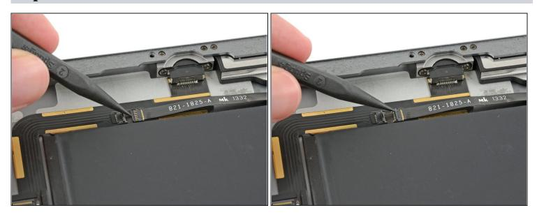
• Use the pointed end of a spudger to flip up the retaining flap on the left speaker cable connector.
