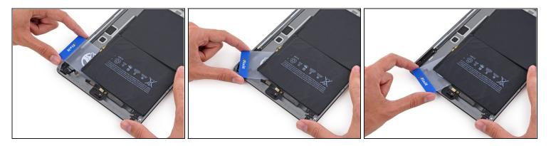
Slide the card around the upper right corner of the battery.
