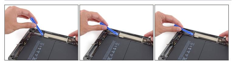
• Pry up the logic board at the lower edge of the rectangular gap, near the EMI shield.
