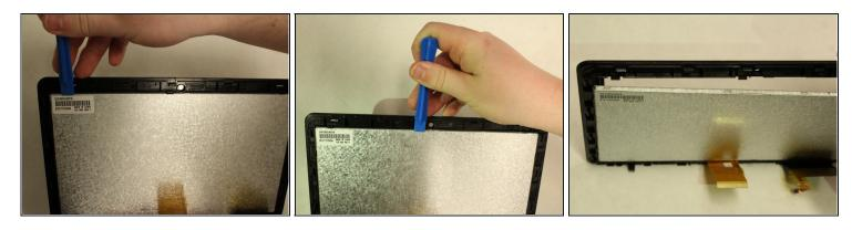
• Continue to slide the opening tool along the length of the casing until there is a clear separation between the screen and the cover (as shown in the third image).
