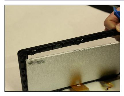
Once there is a clearing, carefully remove the screen from the black cover. You now have separated the screen from the tablet device and and are now ready to replace screen.
