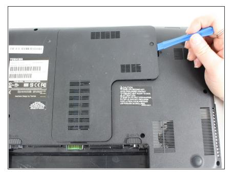
Use the plastic opening tool to pry the panel open. Be sure to do this on all four sides. Then the panel will lift off.
