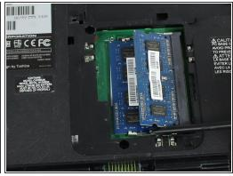
Take the nylon spudger, and push the prongs so that it releases the RAM.
