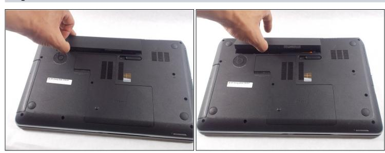
• Lift the battery up out of its socket.
