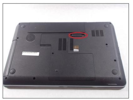
• Push the lever underneath the battery to the left.
