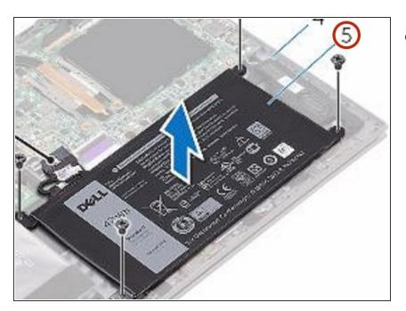
Lift the battery off the palm-rest assembly.
