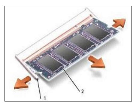
Slide the **NEW** module firmly into the slot at a 45-degree angle, and rotate the module down until it clicks into place. If you do not feel the click, remove the module and reinstall it.
