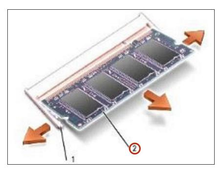
Remove the module from the connector.
