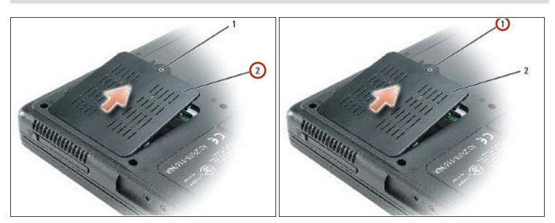
Replace the cover and tighten the captive screw.
