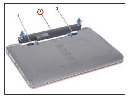
Push the battery in place till it snaps into place.
