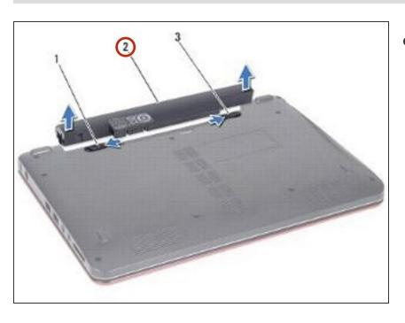
Pull the battery up and out of the battery bay.
