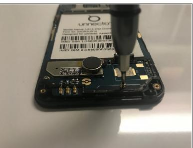
Use a Phillips #000 screwdriver to remove the four screws that secure the motherboard.
