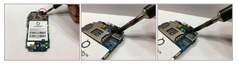
Desolder the headphone jack using a soldering iron on each of the 6 points holding it down.
