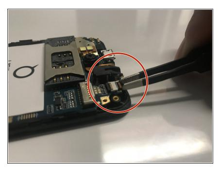
Disconnect the ribbon cable from the motherboard using rounded, spadetipped tweezers.
