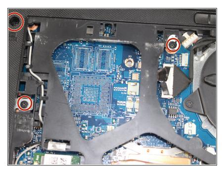
Use a JIS #1 screwdriver to remove the three 7 mm screws.
