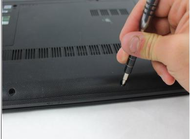
Use a JIS #1 screwdriver to remove the two 7 mm screws.
