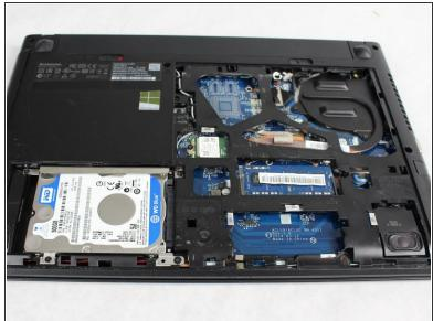
Remove the back panel by sliding it away from the battery.
