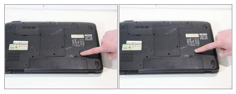
• Unlock the battery by flipping a switch near the release latch.
