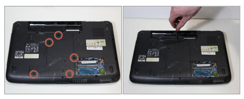
Unscrew the 2 captive screws and 3 M2.5 x L8 screws holding back cover in place.
