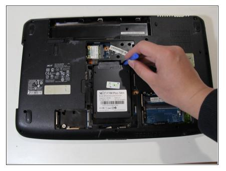
Using an opening tool or your hands, slide the hard drive out of its connector.
