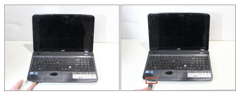
Press in the SD Card or the SD Card Dummy if no SD Card is there. Remove card when it pops out.
