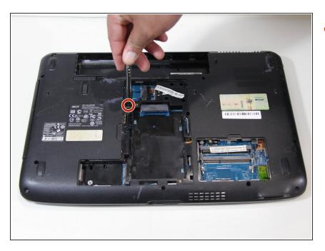
Remove 1 M2 x L4 screw holding the drive in place with a screwdriver.
