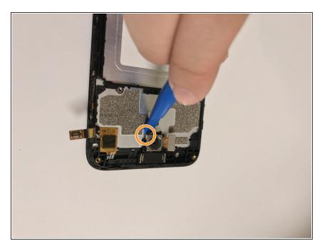
Gently put the opening tool head as close as possible to the edge, where the camera and the phone stick.
