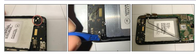
• Remove both of this cables located on the bottom left corner of the phone.
