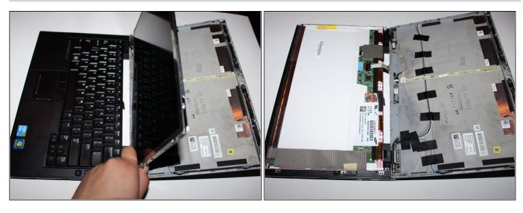
• Carefully lift the screen up and flip it over onto the keyboard side as if you were turning the page of a book.
