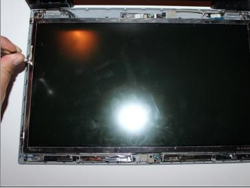
• Remove the six 0.3mm Phillips #1 screws.
