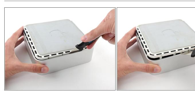
Keep working around the perimeter, freeing the clips along the final edge.
