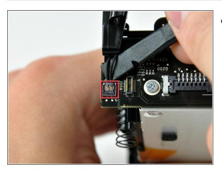
Use the flat end of a spudger to pry the hard drive thermal sensor cable connector up off the interconnect board.
