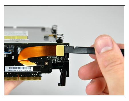
Use the flat end of a spudger to pry the audio ribbon cable connector up off the interconnect board.
