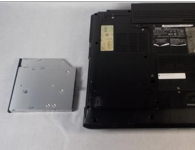
Pull the Optical Drive firmly out from its slot to remove it from the laptop.
