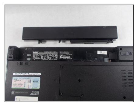
Remove the battery from the slot.
