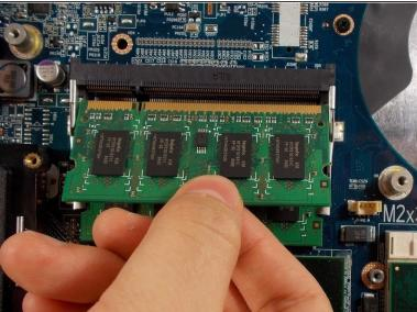
Pull the top piece straight out of the socket.
