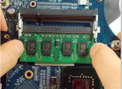
• Repeat the same process by pushing the bottom metal tabs outward and away from the RAM.
