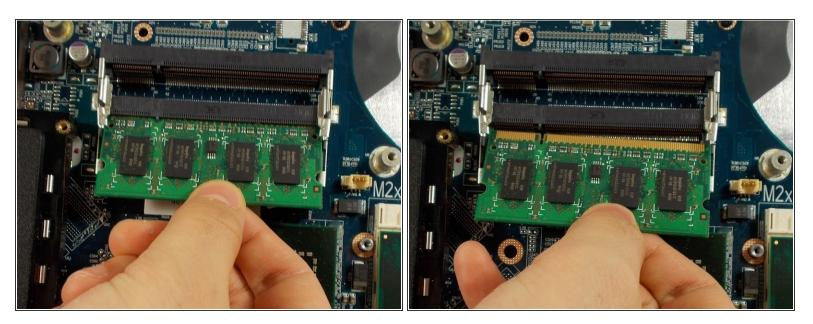
Pull the bottom piece straight out of the socket.
