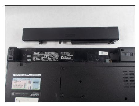
Remove the battery from the slot.
