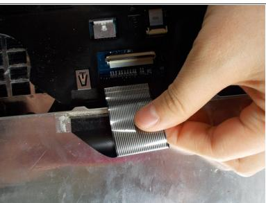
Pull directly outwards to remove the keyboard completely.
