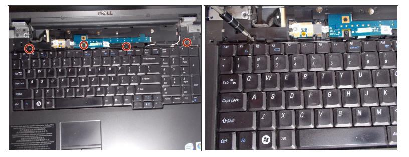
Remove the four 3mm Philips #1 head screws.
