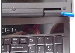
• Use the plastic opening tool to loosen the plastic hinge cover that is located above the keyboard.
