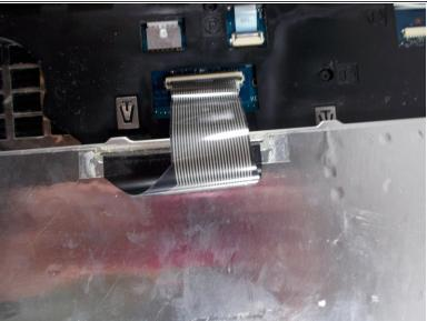
Lift the black tab that the keyboard is plugged into.
