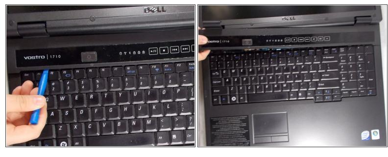
Remove plastic hinge cover by gently lifting up the cover with a plastic opening tool from one side to the other.
