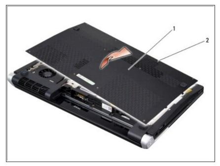
Loosen the ten captive screws on the base cover and lift the cover off the computer at an angle as shown in the figure.
