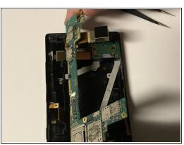
• Use a spudger to pry up the bottom end of the motherboard, then pull it out.
