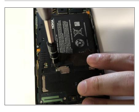
Remove the 4mm Torx #4 screw that's securing the battery connector.
