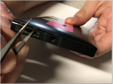
Place tweezers or an opening tool in the SIM card slot and push upwards until the back panel pops out.
