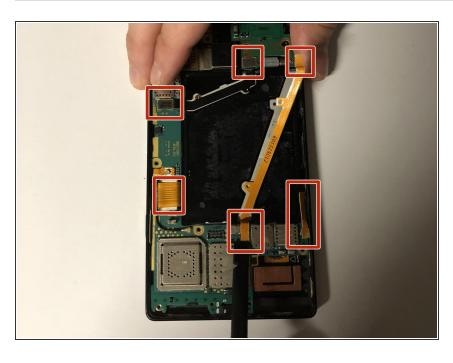
Use the flat end of a spudger to disconnect the six ribbon cables from the motherboard.
