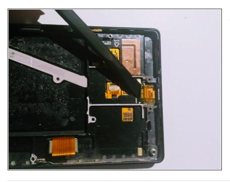
Use spudger to remove 3rd microphone. Located on the last layer before the display screen.
