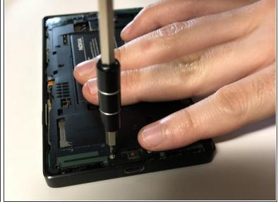
• Remove all ten 4mm Torx #4 screws that secure the battery cover to the frame of the phone.
