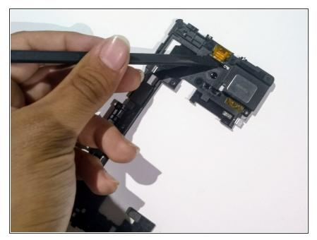
Use spudger to remove 3rd microphone. Located on the engine board cover.
