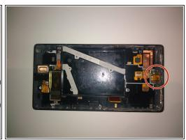
Locate all microphones. The first two microphones you will find are on the engine board. The two microphones will be back to back with each other. The third microphone will be on the engine cover. The last microphone will be on the last layer of the phone before the screen.
