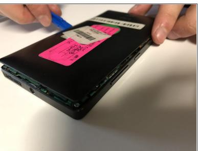
Wedge a plastic opening tool between the two panels. Slide it along each side of the phone to completely remove the back panel.
