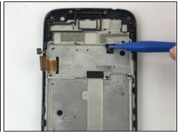
• Peel up the small tape that's connected to the screen with a plastic opening tool.
