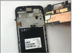
• Using the plastic opening tool, carefully pry up the motherboard.
