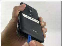
• Open case with a plastic opening tool that has the same size as the divot located at the bottom left of the phone. If you don't have an opening tool, use your finger nails.
