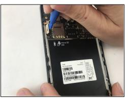
Using an opening tool, pry up one of the connectors to the left of where the sim card was located.
