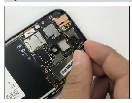
After detaching the connector, carefully remove the camera using tweezers. If you don't have tweezers, use your hands.
