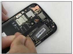
• Use the flat end of a spudger to disconnect the rear-facing camera connector from its socket on the mother board.
