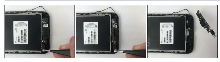
• Insert the tweezers under the vibrator and gently lift up the whole part.
