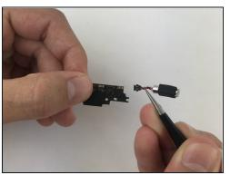
• Pop up on the vibrator's connector to separate it from the charging port.
