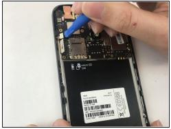
• Pry up the next connector located right on top of the previous one.
