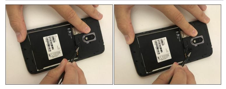
• Remove the small silicon cover at the bottom right of the camera using <u>tweezers</u>.
