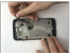
• Peel the flexible black cable using a plastic opening tool and or your fingers.
