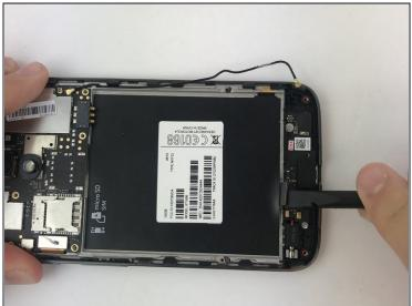
• Use the flat end of a spudger to pry up on the connector at the bottom of the battery space.
