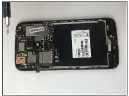
• Using the Phillips screwdriver, remove the screw that's found next to the speaker on the top left of the phone.
