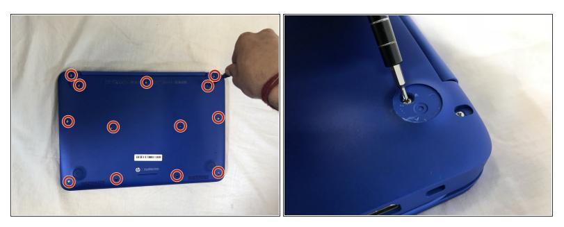
Remove the thirteen 5mm Phillips #0 screws from the bottom case.
