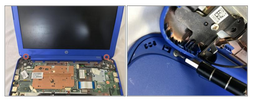
• Remove the two 5mm Phillips #0 screws from the screen bezel.
