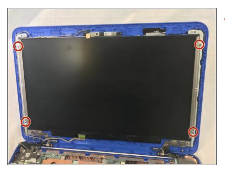
Remove the four 3mm Phillips #0 screws from the screen.
