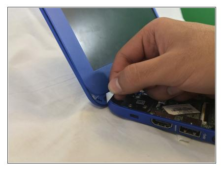
• Remove the screw covers from the bottom corner edges of the screen.
