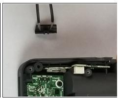
• Use tweezers to lift the power switch out and set aside.
