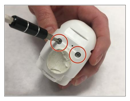
Remove the 2 (.135") housing screws with a JIS00 screwdriver
