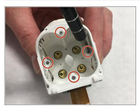
Remove 4 (.135") screws on the inside of the battery compartment using the JIS 00 screwdriver.
