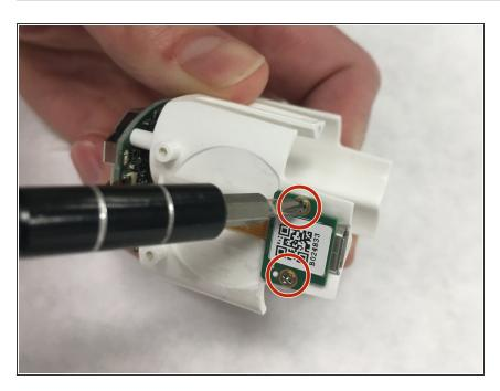
Remove the 2 (.135") screws holding the charging port on using the JIS 00 screwdriver.
