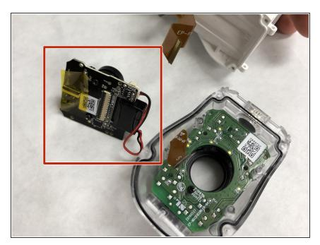
Once all ribbon cables are removed, remove the motherboard and camera assembly by pulling up on the black camera motherboard.
