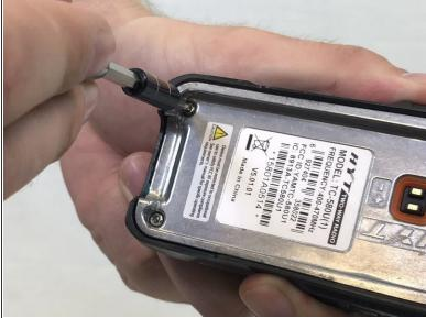
Remove the two 15mm T8 Torx screws from the base of the battery cavity.
