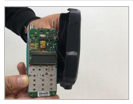
If not already done, remove the circuit board completely from the case.
