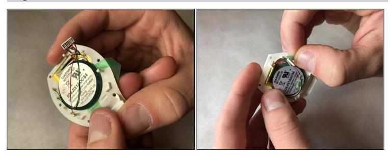
• Remove the green tape shrouding the battery connector.
