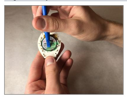
On the back cover use a plastic opening tool to remove the green tape retaining the battery.
