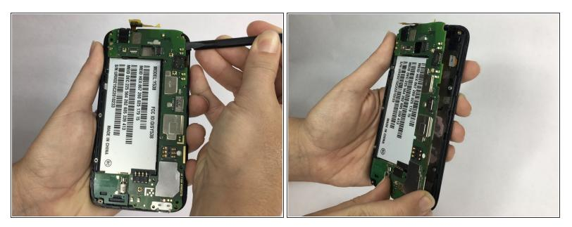
Wedge the flat end of a spudger underneath the motherboard and pry upwards to separate it from the frame.
