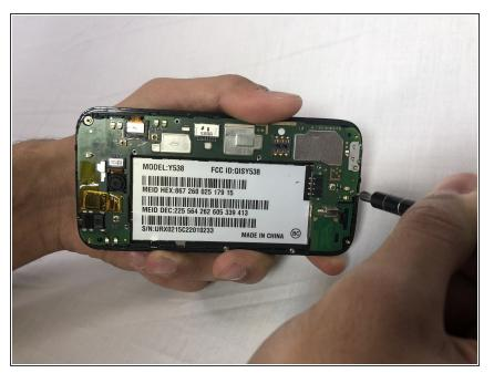
• Remove a single 3mm Phillips #00 screw from the motherboard.
