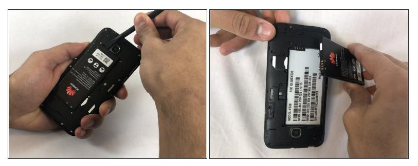
• Use the flat end of a spudger, or fingernail, to lift up the battery and pull out.
