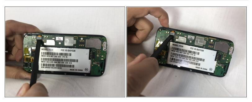
• Using the flat end of a spudger to disconnect the motherboard ribbon cable.
