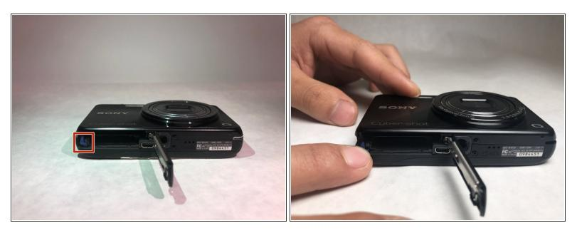
• Pull down on the blue tab to release the battery.
