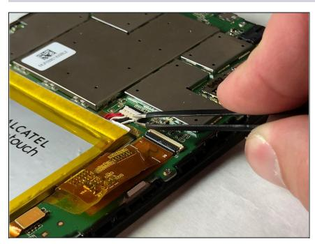
Disconnect battery by pulling up on the ZIF connector with precision <u>tweezers</u> for safety.
