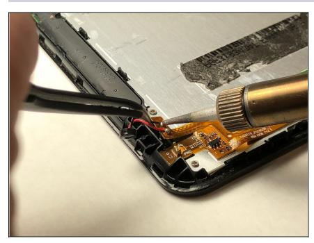
Solder the wires off of the motherboard with a soldering iron while holding the wires with the precision tweezers. For information on how to solder safely and correctly go to this link: How To Solder and Desolder Connections
