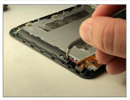
Remove the Microphone from it's slot with the precision tweezers.
