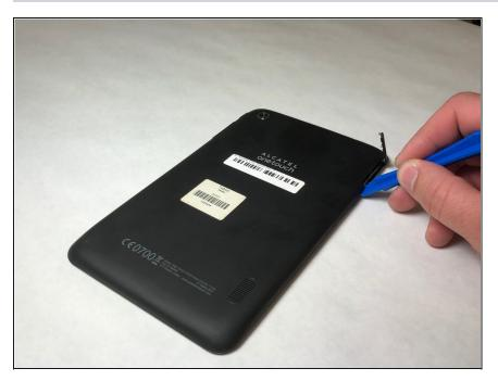
Use the plastic opening tool to pry around the edges of the back cover until it pops off.
