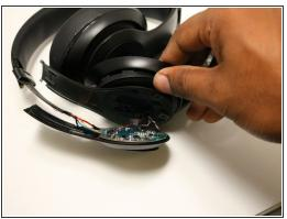
Pass wire through new housing and reconnect wires.
