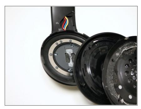
Pull secondary housing away gently being careful not to damage the wires.
