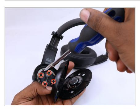
Remove four screws using a Phillips head screwdriver to remove the third housing.
