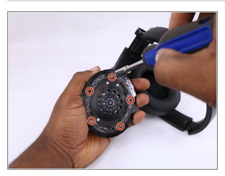
Remove five screws using a Phillips head screwdriver from speaker housing.
