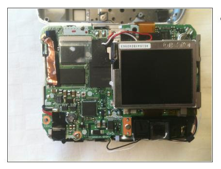
Remove the two screws on the top edge of the circuit board to the right of the viewfinder.
