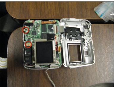
Remove the two screws on the top edge of the circuit board, to the right of the viewer.
