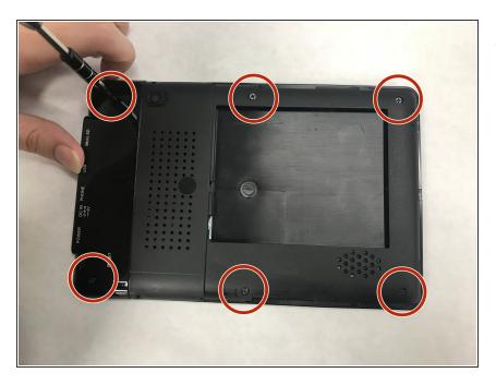
Unscrew the six 6.01mm Phillips one screws that hold the casing together.
