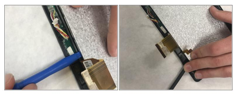
• Pry the screen open with the blue plastic opening tools while using another plastic opening tool as a jack to remain in place while you pry around the entire screen.
