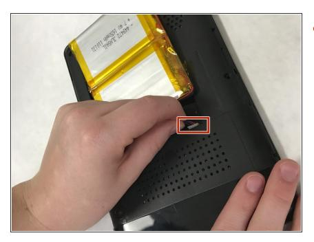
Pull on the plug carefully until it releases from the port and simply pull the battery out after.
