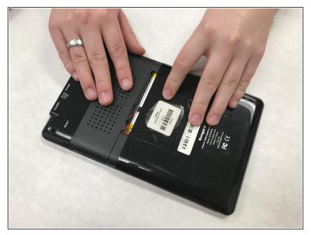
Press firmly on lower portion of the back cover and slide the cover towards the bottom to remove cover.
