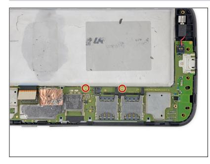
• Use a T3 Torx driver to remove the two bronze-colored, 2.4 mm screws securing the motherboard.
