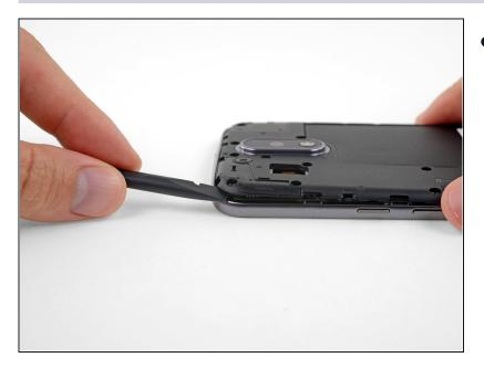
• Insert a spudger under the midframe at the top left corner, and gently twist to separate it from the body of the phone.
