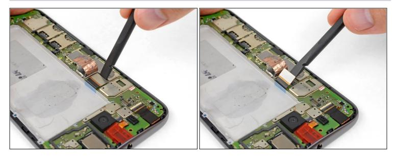
• Use your spudger to disconnect the display by prying its connector straight up from the motherboard, on the edge nearest the side of the phone.
