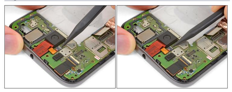
• Pry up with your spudger to flip open the locking flap on the headphone jack's <u>ZIF</u> <u>connector</u>.
