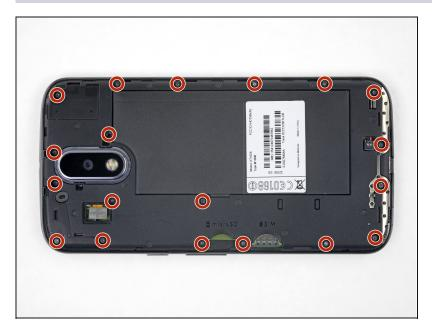
• Use a T3 Torx driver to remove the nineteen identical 3.1 mm screws securing the midframe.
