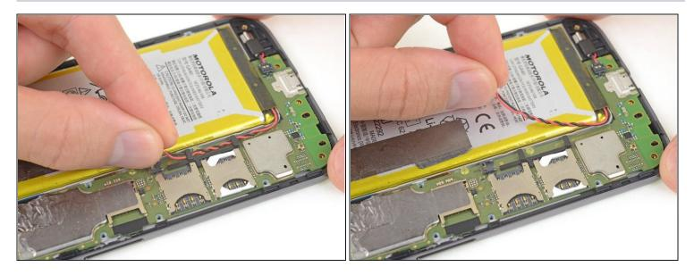
• Peel off any tape securing the battery wires, and then push the battery wires towards the battery to de-route them from the black bracket on the motherboard.
