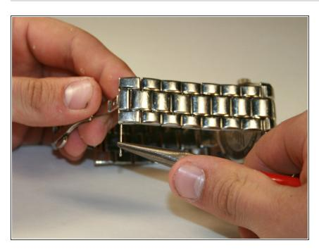
Use your pliers to pull the pin the rest of the way through.
