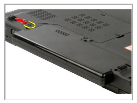
Slide the battery lock latch on the left away from the battery.
