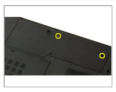
Remove the two screws that secure the hard drive and mini-card access panel to the computer.
