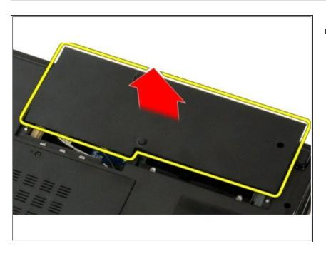
Remove the hard drive and minicard access panel.
