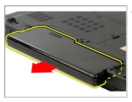
Slide the battery itself toward the back of the computer and remove
