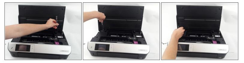
• Unscrew and remove the bottom 13mm TR10 Torx Security screws using the iFixit screwdriver
