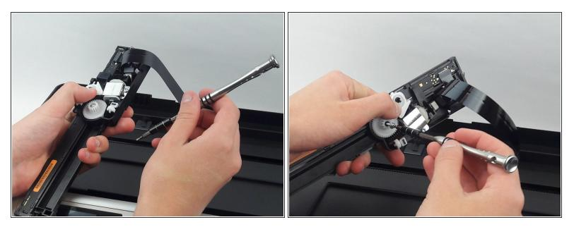
Unscrew and remove the 13mm TR10 Torx Security screw in the center of the gear using the iFixit screwdriver
