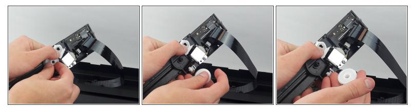
• Locate the white gear and remove.
