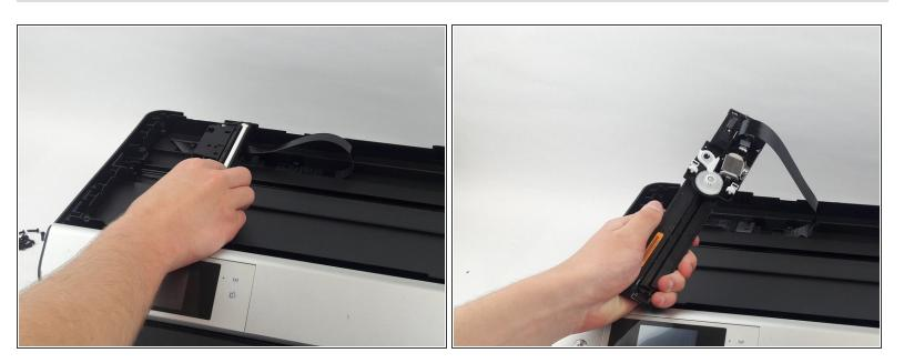
• Locate the Scanner Arm Accuator and remove.
