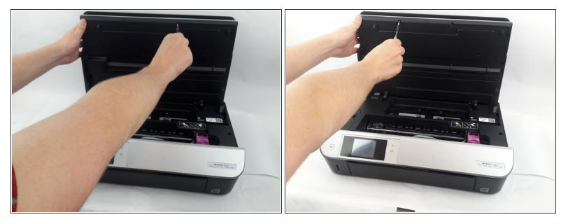
• Unscrew and remove the upper 13mm TR10 Torx Security screw using the iFixit screwdriver
