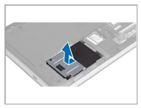
Slide the hard drive in the direction shown and lift the tab to remove it from the computer.
