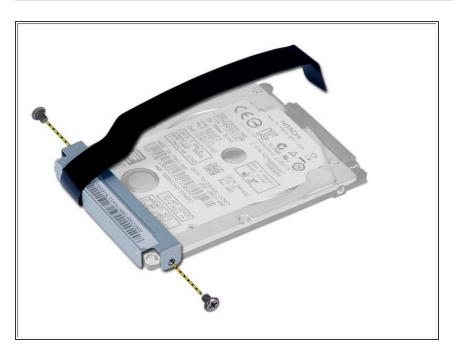
Remove the screw that secures the hard-drive caddy to the hard drive and remove it.
