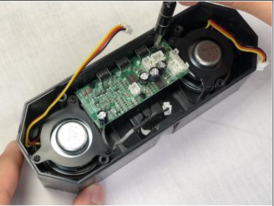
• Remove the three 9.1mm Phillips #1 screws located on the circuit board.
