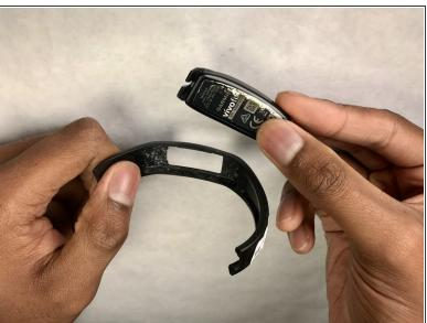
Carefully peel back the wristband so the bottom of the device is facing you. Then, pull out the
