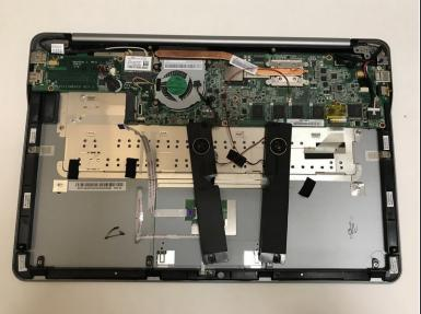
Pull off the black strips of tape from the speaker wires and remove the speakers from the laptop.
