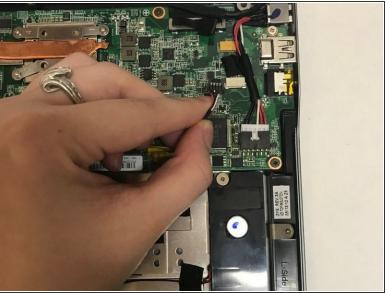
Unplug the wire connecting the speakers to the motherboard.
