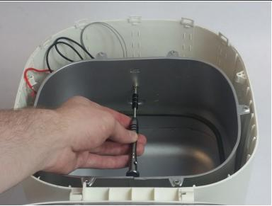
Remove the single 11mm Phillips #1 screw thats holding and inner lining in place.
