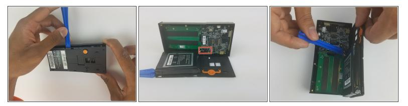
• Pry open the back case as shown using the Plastic Opening Tool.
