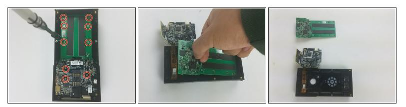
• Unscrew the 9 1 mm screwdrivers using a PH00 Phillips Screwdriver.
