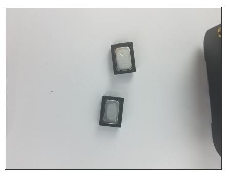
• To remove the speakers pry each one out carefully with a plastic opening tool.
